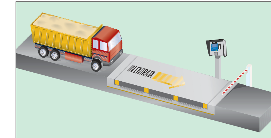
Unmanned weighing. The vehicle enters and drives onto the weighbridge, always in the same direction.
